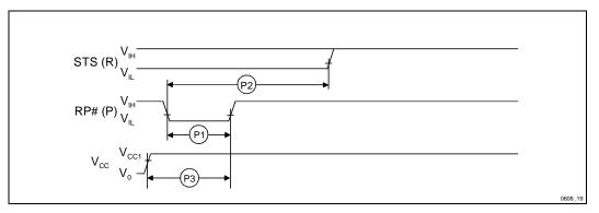
Figure 19. AC Waveform for Reset Operation
