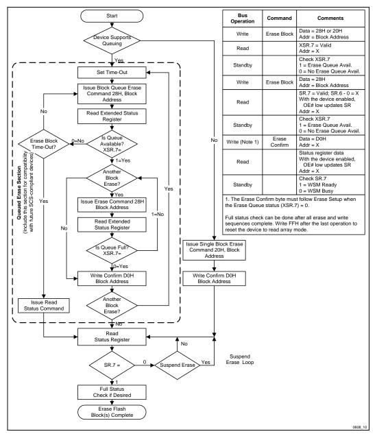
Figure 9. Block Erase Flowchart
