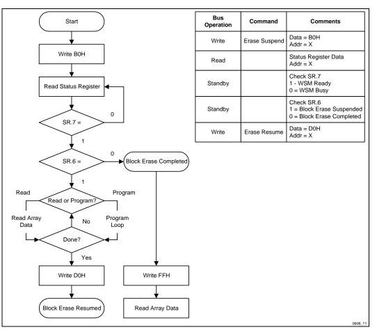
Figure 10. Block Erase Suspend/Resume Flowchart
