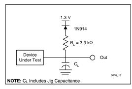
Figure 16. Transient Equivalent Testing Load Circuit
