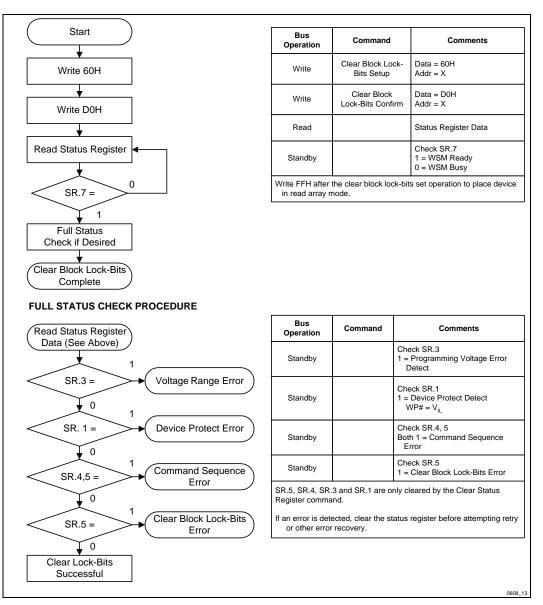
Figure 12. Clear Block Lock-Bits Flowchart
