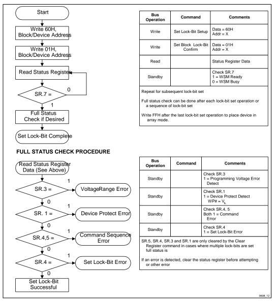
Figure 11. Set Block Lock-Bit Flowchart
