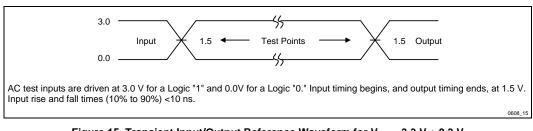
Figure 15. Transient Input/Output Reference Waveform for V<sub>CC</sub> = 3.3 V  $\pm$  0.3 V (High Speed Testing Configuration)
