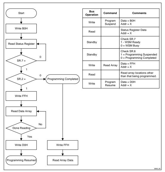
Figure 8. Program Suspend/Resume Flowchart
