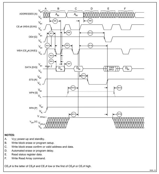
Figure 18. AC Waveform for Write Operations
