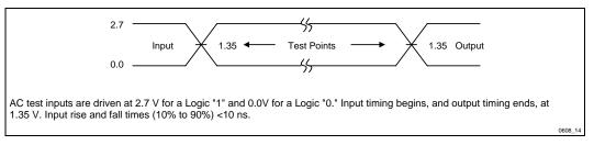
Figure 14. Transient Input/Output Reference Waveform for V<sub>CC</sub> = 2.7 V–3.6 V
