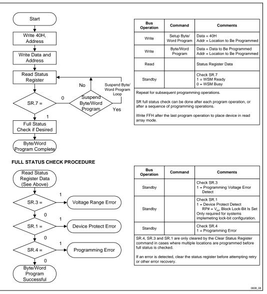
Figure 7. Single Byte/Word Program Flowchart
