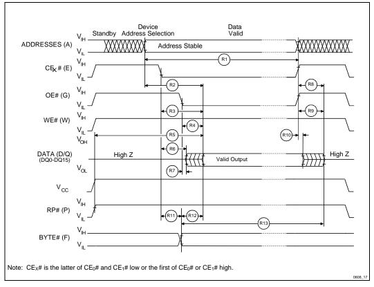
Figure 17. AC Waveform for Read Operations
