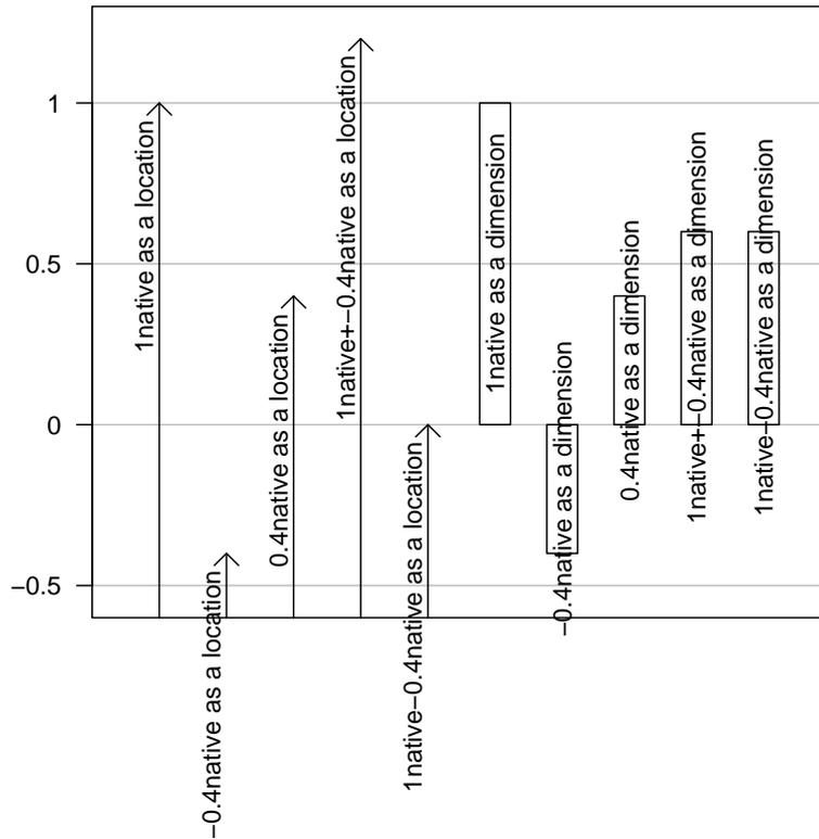
2. The functions `convertX`, `convertY`, `convertWidth`, `convertHeight` are used to convert from one coordinate system to another. Again, it is important whether the conversion is for a location or for a dimension. The following code demonstrates some results from these functions based on a similar situation to that in the preceding diagram:
